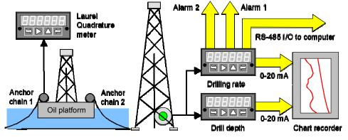
Once drilling has begun, there is the additional challenge of accurately measuring the length of drilling shaft that has been sunk into the seabed and reading out the rate of drilling in feet per hour as the drill makes it way through different layers of sedimentary rock. High vibration would give false counts with conventional pulse counters.
