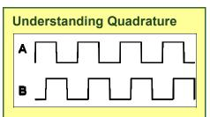
A quadrature signal consists of two square waves A and B that are 90° out of phase. The phase transitions specify direction to allow dynamic up/down totalizing.
