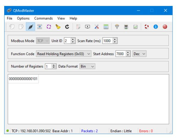
The QModMaster Bus Monitor window presents the Modbus Command transmitted to the LWIFI and its response. Note that the hexadecimal byte values of **00 05** represent the same alarm and overload status shown above in binary.
