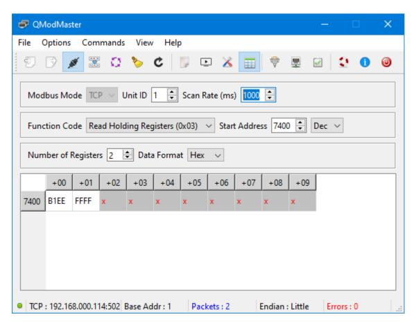
The QModMaster Bus Monitor window below presents the Modbus Command transmitted to the LWIFI and its response. Note that the hexadecimal byte values of **B1 EE FF FF** represent the 32-bit signed two's complement display value. The four bytes are combined as **FFFFB1EE** to form the 32-bit value which is -19986 decimal. A condensed description of two's complement is available on Wikipedia.
