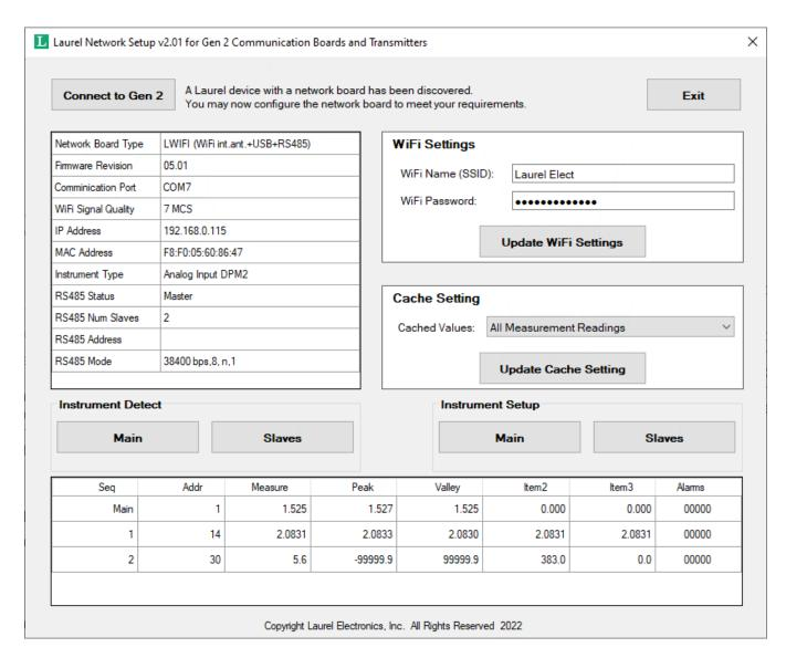
The LNET1485 board does not have a mini-USB connector but an RJ11 connector for RS485. That connector can be used for setup using Laurel Network Setup (LNS) software or Instrument Setup (IS) software, and for data transfer with an RS485 bus with a mix of up to 31 Laureate meters and transmitters.
