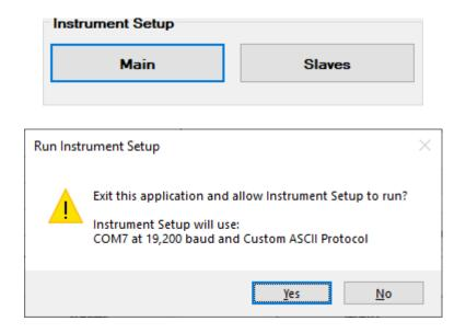
In the "Communications Setup" screen of IS software, select the "Custom ASCII" protocol, click on "RS485 Full Duplex," and click on "Yes" to indicate that there is only one meter on the RS485 bus.
