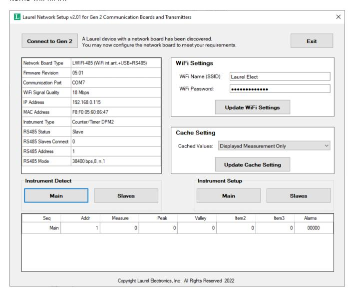
Click on Main under "Instrument Detect" to update the LNS screen and delete previously discovered items which do not apply.
