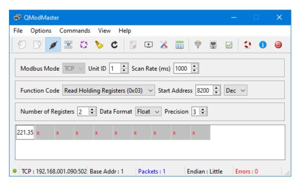
The QModMaster Bus Monitor window below presents the Modbus Command transmitted to the LWIFI and its response. Note that the hexadecimal values of **59 9A 43 5D** represent the value in IEEE 754 floating point format (little endian). See Wikipedia for a condensed description of IEEE 754.
