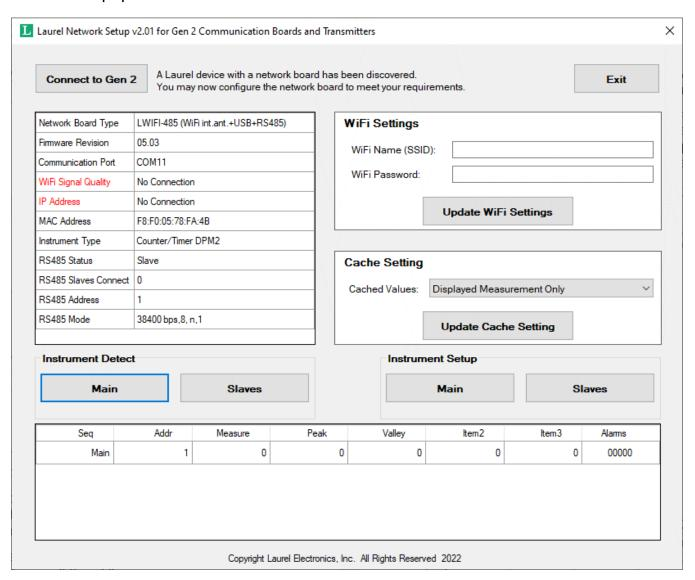
The LNS screen will now show the Network Board Type, the COM port used by the PC, and the MAC address of the WiFi chip. At this point the IP Address and WiFi Signal Quality are still shown as "No Connection."
