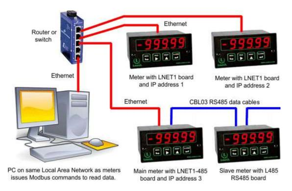
**LNET1 & LNET1485** allow a Laureate meter, counter or timer to be plugged into the same wired LAN as a PC or HMI that serves a Modbus Master. As or WiFi, devices by different manufacturers can be on the same network and are addressed by their IP address. That address is typically assigned by the router, but with LNET1 and LNET1485 it can also be entered by the user with our Laurel Network Setup (LNS) software, as explained in this manual.
