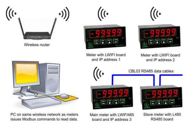
**LWIFI & LWIFIX** operate the same, but LWIFI has an onboard printed antenna while LWIFIX comes with an external antenna and a 30" (76 cm) antenna cable. The external antenna is designed for mounting on the top surface of a metal cabinet that would block the radio signal of the onboard antenna. It also provides greater range than the onboard antenna.
